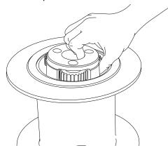
5. Remove the other four capscrews and lockwashers holding the tieplates to the bearing support endplate. Remove the planet assembly from the drum and separate the drum from the bearing support endplate.
